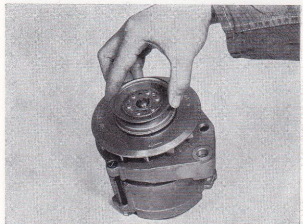
Fig. 51. Removing the pulley
