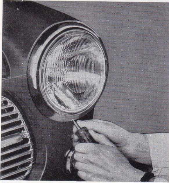
Fig. 113. Removing the headlight rim
