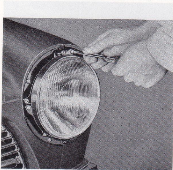
Fig. 114. Removing the holding ring
