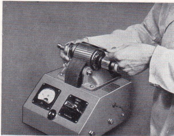
Fig. 9. Testing the armature
